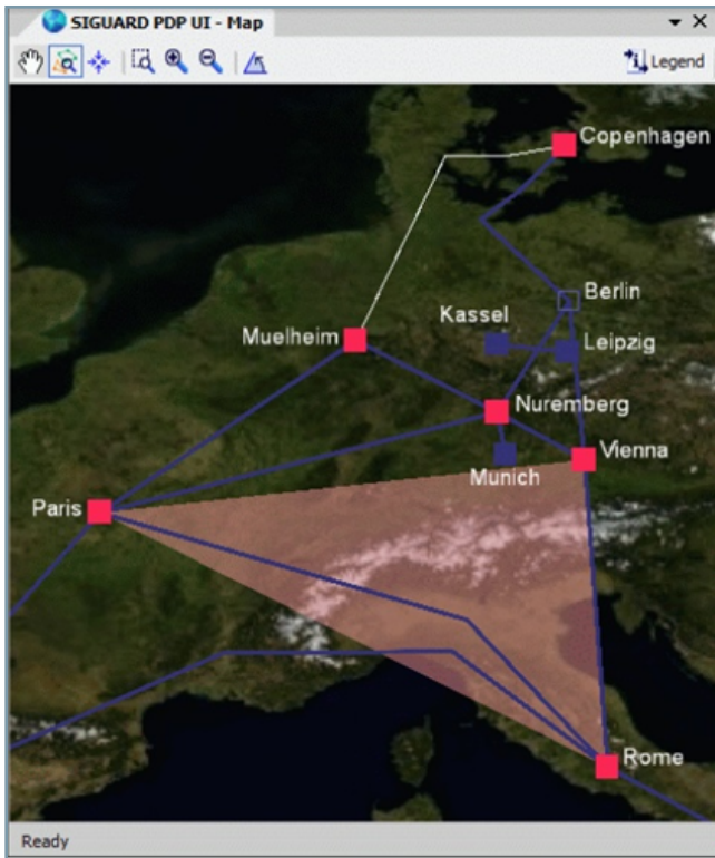
Figure 6.3/8 Visualization of a Detected Short-Circuit A Red Triangle Connects the 3 Stations Most Affected by the Short-Circuit
